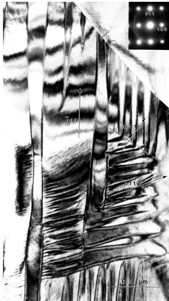
Figure 9. BF micrograph showing the complex domain configuration of PZT45 ceramics (grain viewed along [0\bar{1}1] ).
