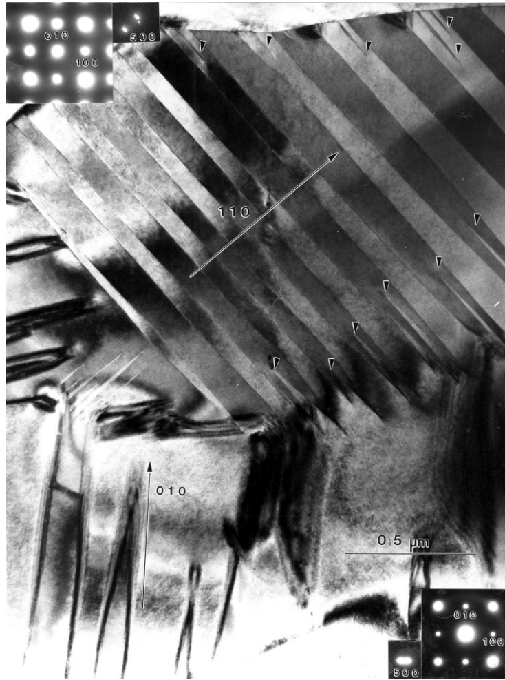
Figure 8. BF micrograph showing the mixture of two different types of domain configuration in PZT45, viewed along [001] . The insets show the selected-area diffraction patterns of the region of domain bands (top) and of wedge-shaped domains (bottom). The (500) reflection is enlarged to show the splitting of the spot.
